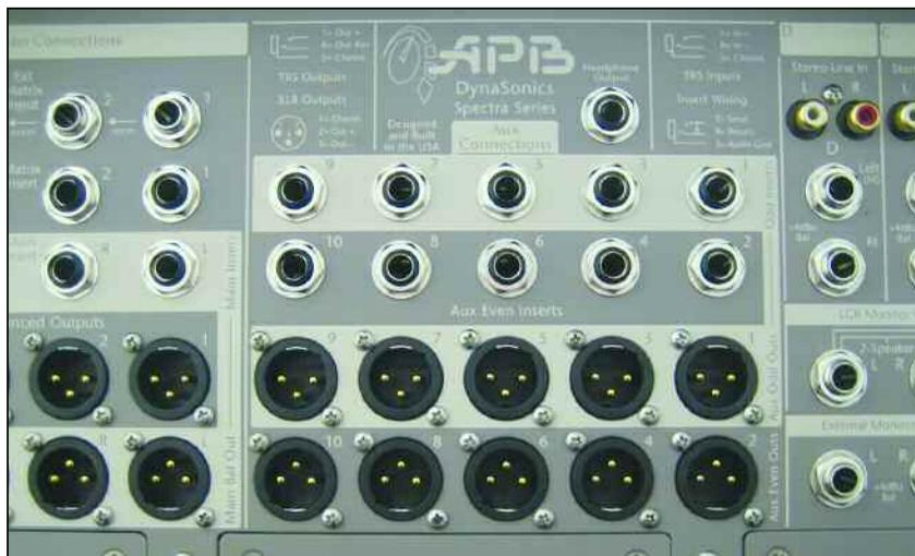
*The Aux outputs offer pre/post assignment to matrix section and assignments to left, right, center and mono buses.*
