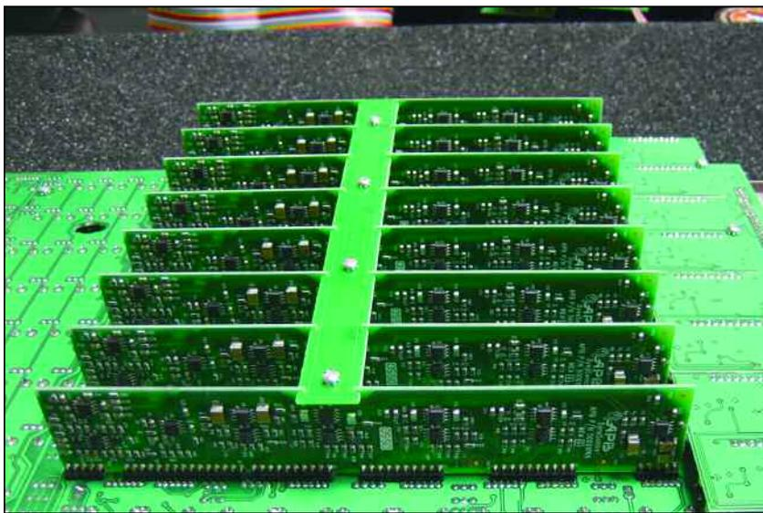
The EQ boards in place on the main board, and each can be easily swapped out if required.
