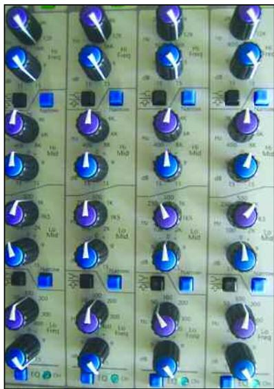
*The Spectra-T EQ is sweepable in all four bands and includes shelving/bell switches on both HF and LF bands.*
